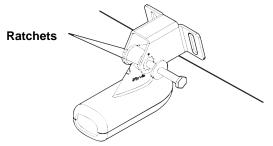
Insert bolt and check transducer position on transom.
